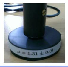
In order to check the calibration the permeability probe is placed perpendicularly on the top of the standard so that the tip touches its center. The measured value should correspond with the number printed on.
